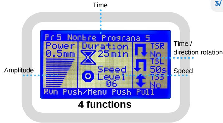
Adjustment of 4 different parameters with only one command and LCD screen which allows access to all information during sieving
